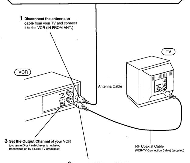
2 Connect the VCR to your TV with the RF Coaxial Cable (OUT TO TV).
